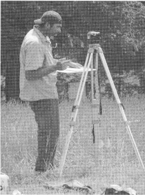
Archaeologist Andy Beupre uses a transit to position test pits during the dig on June 6 and 7 at the original site of the Orleans County Grammar School on Prospect Hill.
