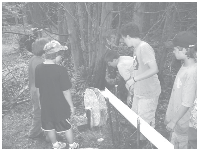
The Water Power group tested the wheels they built on Friday at the Time Travelers Day Camp. Earlier in the week they had diverted a portion of the stream just beyond our pasture with a sluice they made using rain gutters supported by stakes. They tried both overshooting and undershooting the stream of water, and counted the revolutions per minute to see which was faster.
